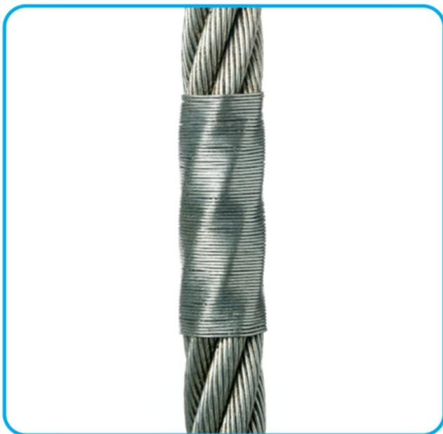
Figure 1: Seizing of wire rope.
