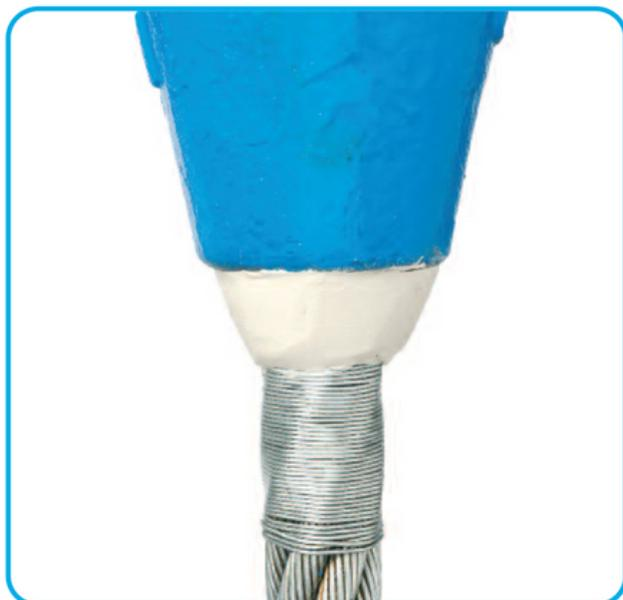
Figure 7: Axes of socket and rope properly aligned and sealed with **WIRELOCK**<sup>®</sup> putty/ clay.
