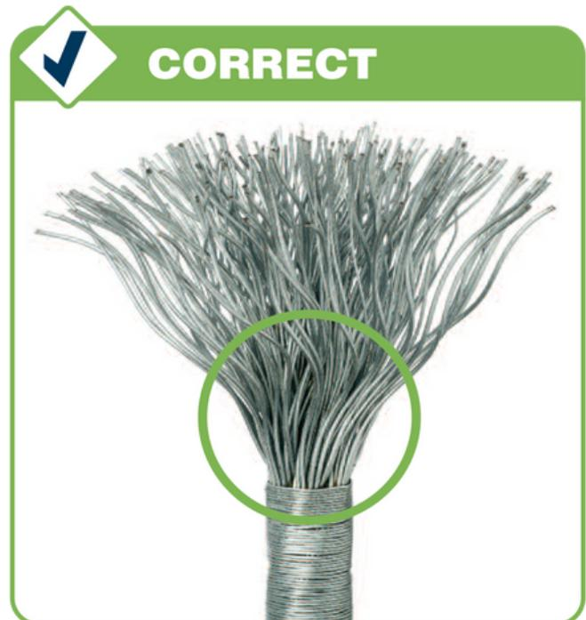
Figure 3: Properly broomed wire rope unlaid from the end of the rope to the seizing.
