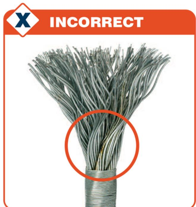
Figure 4: Incorrectly broomed wire rope.
