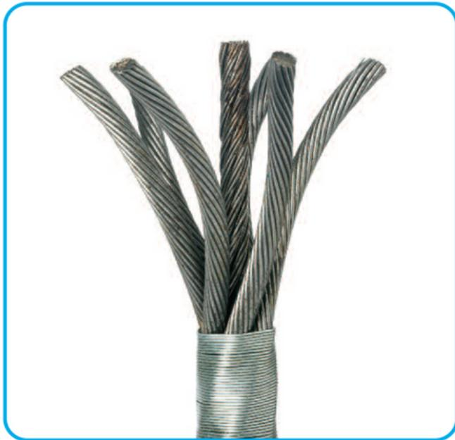
Figure 2: Unlay wire rope so that the angle does not exceed 90°.
