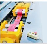
All synthetic webbing products are tested in-house using our calibrated pull testing machine.
