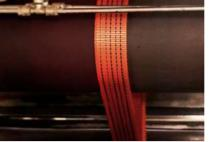
All Petrolift slings are colour and line coded according to industry standards to indicate safe working load limit.
